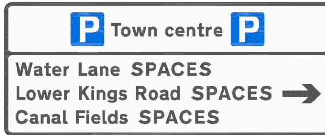
Figure 7 Example High Street West VMS Sign
